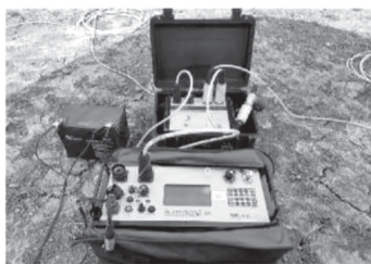
Figure 4: Groundwater exploration by using surface geophysical survey (Electrical resistivity methods)
